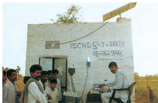
Fig. 5.10: Solar operated electronic milk testing equipment
