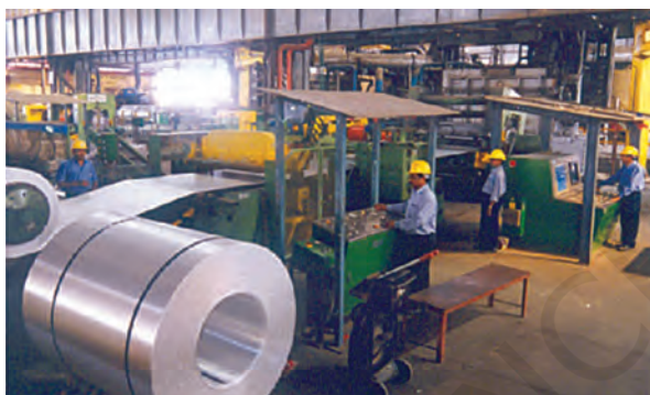
Fig. 6.3: Strip casting mill at smelter of NALCO
